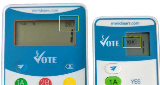
Figure 5 - "OK" indicates that your vote has been received by the base receiver
