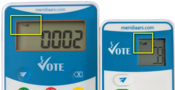
Figure 3 - Signal strength depends on the distance of the keypad from the base
