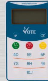
Wireless keypad (clicker) uses a proprietary communication protocol to send data entered by the student to the USB base receiver.
