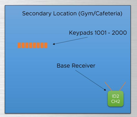
Each Base must be configured to a different ID and Channel and assigned a unique segment of the keypad range. Both must be connected to the same computer to collect the votes at the same time.
